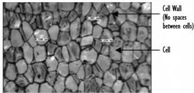
**Figure 2: Expanded Polystyrene Cell Structure**
